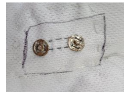
Figure 1. CNT-coated thread mechanomyography (MMG) sensor sewn pattern
