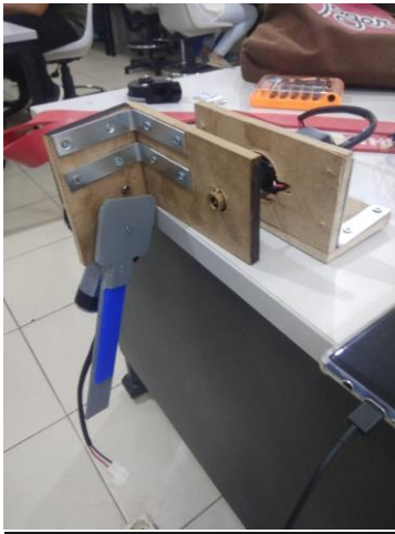
Figure 14. Arm support design with universal power window proof of concept model
