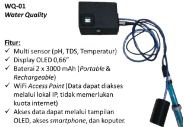
Gambar 1. WQ-01: Sistem Monitoring Kualitas Air (PH, Temperatur, Kekeruhan, TDS)
