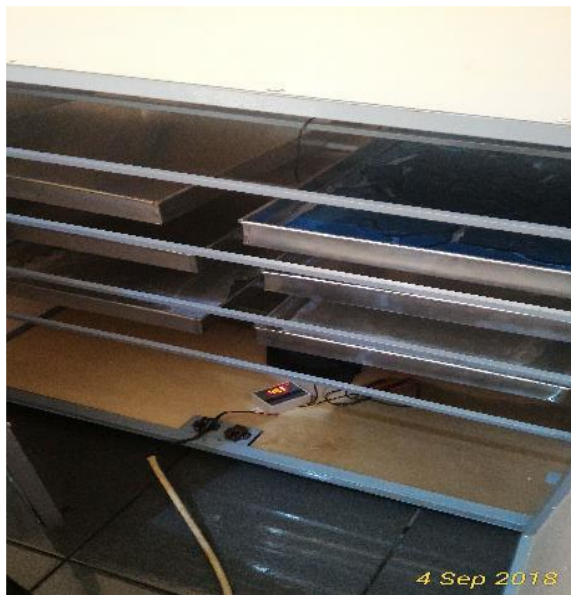
Gambar 2 Prototipe oven pengering indigo powder skala 5 kg perhari
